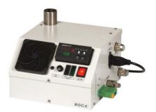
Due to its innovative technology, it can be used for numerous applications, and it is very economical to run - only -98W/h of electrical input for 1kg of humidity. The adiabatic humidification principle receives energy from the warm air and cools the object to be humidified (cooling by evaporation) with simultaneous reduction of the operating time of the cooling units. Both factors ensure that UB1-4CT pays for itself in a very short time.
