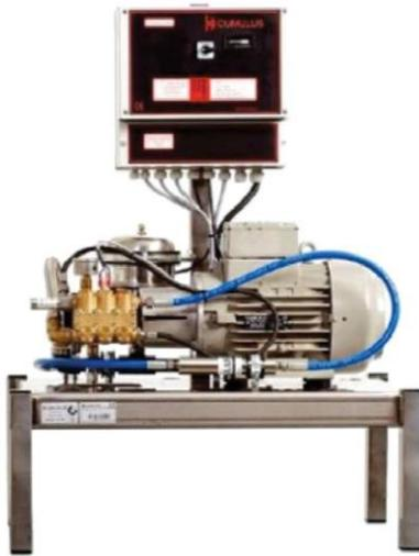
The High-Pressure Booster Min Is a high-pressure humidification unit without reverse osmosis unit. The unit has its own control unit, therefore it can operate stand alone, if required, the unit can also be connected to a Building Management System to control it. Standard version is MIN type. The capacity range is 60 Lt/h, and 800 Lt/h. Pumps can be mounted on stainless steel surface. One control unit, status display and operating hour counter can mount on a unit directly.
