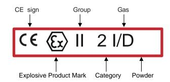
Evolution no-smoke Atex arms are designed in accordance with Directive 98/37/EC and Atex Directive (94/9/EC). The classification of the arm is as above according to ATEX rules.
