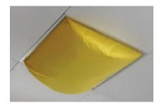
DiffuSox™ air diffuser is made of metal frame and highly permeable fabric, the air dispersion surface attach to the metal frame via Velcro, connecting to metal inlet via square to round fitting and detachable inlet.
