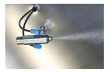
The atomizer nozzle system is a humidification system that can be used in all industrial applications where controlled or constant humidity is required. These humidifiers are used to add moisture to the air by atomizing water or water-based liquids. Compressed air and water are needed for the use of the system. Inside the nozzle, the mixture of air and water is carried out and very small water particles are given to the environment.
